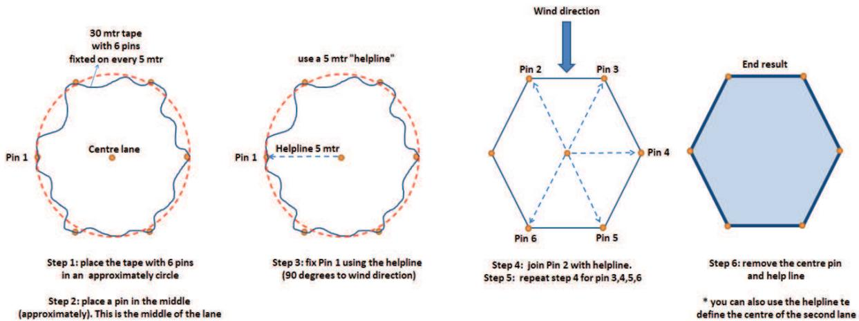
a) The Launch and Landing area is defined using a 30 metre tape pinned around the centre making a hexagon with an outer enclosing circle with a diameter of 10 metres, called the individual “Pilot Area”.
